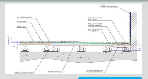
To complete the waterproofing works, Wetrooms UK installed Tilesafe waterproof membrane across the shower floors, finishing 75mm beyond the shower area, and linking 75mm up the walls to comprehensively tank the wet-floor area and ensure there would not be any water ingress into the luxury apartments.
